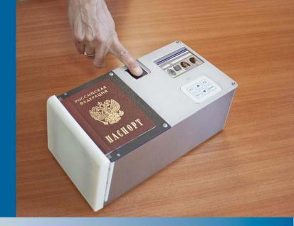
PAPILLON DPP-4 is a compact handheld device with a fingerprint scanner embedded, especially designed for the growing needs in in-the-field identity checks through enquiries to the AFIS databases using subjects' touch fingerprints.
