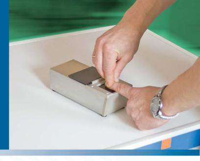
The **DS-22N** is a forensic quality fingerprint scanner manufactured as a separate unit driven by a backbone computer (or a notebook).
