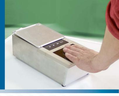
The **DS-30N** is a forensic quality fingerprint scanner manufactured as a separate optical unit driven by a backbone computer (including a notebook).
